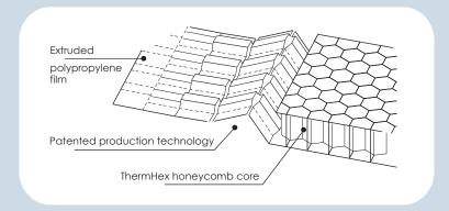
ThermHex honeycomb cores are made with a backing film of polypropylene as standard. This prevents the ingress of resin into the cells during processing, and therefore safeguards uniformity in the mechanical characteristics of the finished component. This also reduces the quantity of adhesive required to the minimum necessary. Polyester fleece layers on both sides are used to finish, achieving a surface for perfect bonding with the core.
